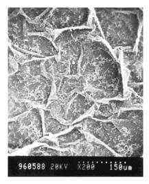
**Figure 1** SEM picture of the PPY film prepared from the system of  $M_{\rm PY}/M_{\rm O} = 1$  and  $M_{\rm O} = 0.2M$ .
